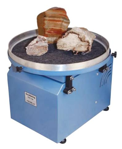
Oscillating Laps are used for flat polishing of slabs, geodes, bookends and clock faces. The oscillating action produces a smoother, flatter surface than can be obtained by hand polishing. We use a heavy steel frame and rugged cast aluminum pans for long, trouble-free operation. Includes polish pan with synthetic pad and separate grinding pan to help minimize contamination. Available in 15" and 20" models.
