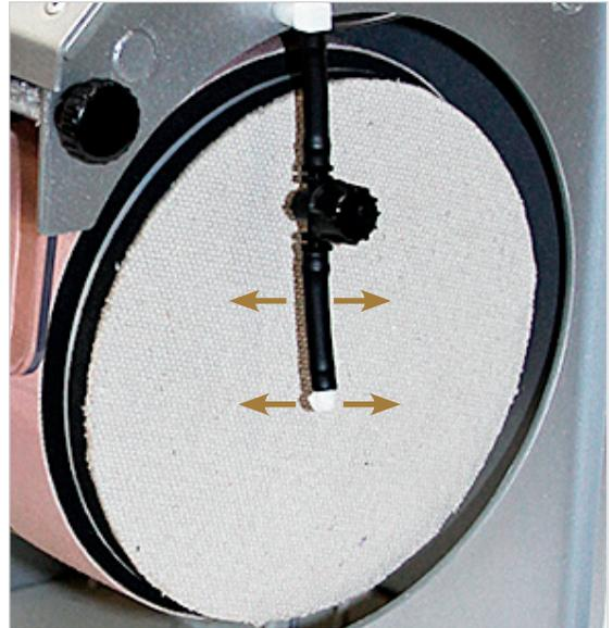
into a jewelry finding, you will need to put a flat on the backside of your cabochon. To do this, attach the included full face diamond lap by screwing it into the end of the right wheel assembly while the machine is turned off. The full face diamond lap must be used with water. Just like the canvas polishing pad, aim the black side spray tube to the center of the disc and adjust the water drip to your preference by moving the black side spray tube and white nozzle to the left or right.
