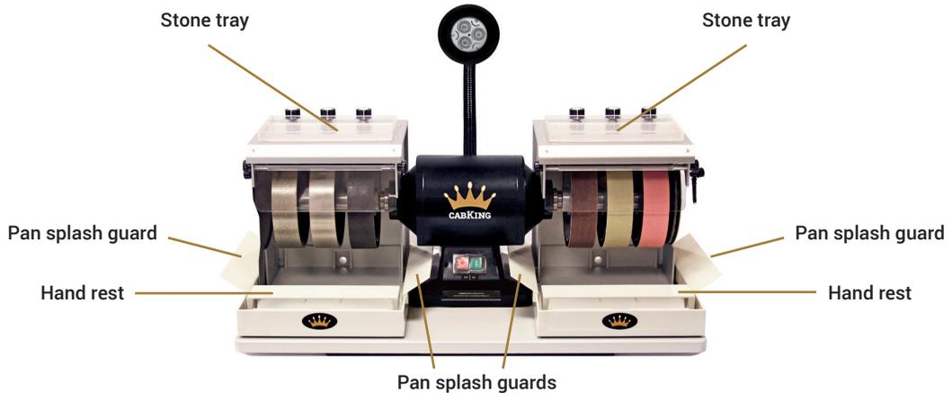
**1** Refer to diagram above for assembly. Determine a suitable, well lit location to place your CabKing-6V3. The machine weighs about 60lbs. You need a sturdy table or stable surface that has 3 feet width by 2 feet depth of clear space.
